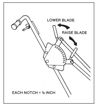
Figure 6, Edger Blade Controls
